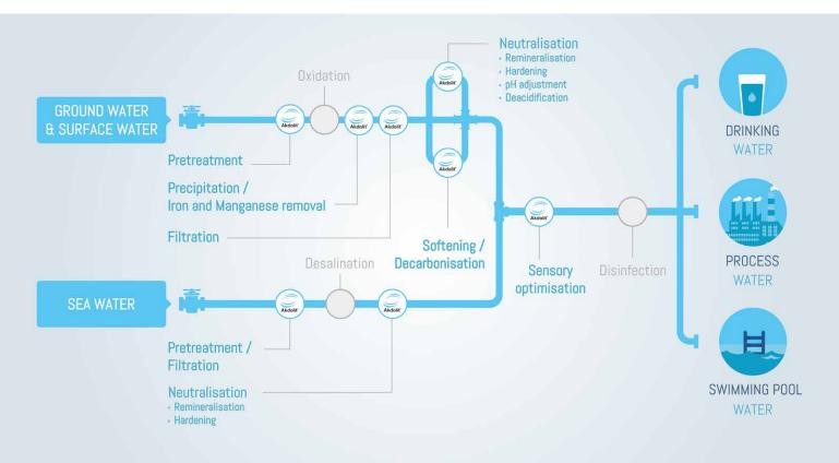
Akdolit® offers an extensive range of reagents and solutions for multiple applications associated with the treatment of drinking, swimming pool and process waters. Our expertise lies in neutralisation, deacidification, mineralisation, hardening, filtration and a number of special applications targeting specific pollutants.
